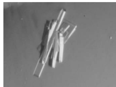
Figure 2 Typical plate crystals of T. maritima TruB obtained by equilibration against a solution of 100 mM citrate pH 3.5, 200 mM Li 2 SO 4 , 20% glycerol, 13% PEG 5000. The maximum dimension of the crystals is about 0.250 mm.
